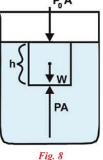
You know that from Newton's law, the net force on it is zero, because it is at rest. What are the forces acting on that water column?
