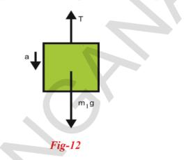
From the FBD of the mass  $m_1$ , there exist two forces on the load of mass  $m_1$ , one is tension of the string acting in upward direction and weight of the load  $(m_1g)$  acting in downward direction.
