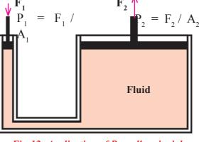
Fig-12: Application of Pascal's principle (bramah press)
