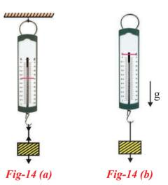
Take a spring balance and suspend it to the ceiling and put some weight to it. Note the reading of the spring balance. Now drop the spring balance with load from certain height to fall freely. Carefully observe the change in the position of indicator on the spring balance scale while it is in free-fall.
