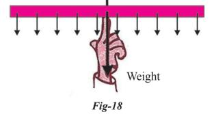
The entire weight of the stick may be thought of as acting at this single point. Hence we can balance the stick by applying a single upward force at this point. • How to find the center of gravity of an object?
