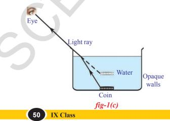
If yes, draw a ray diagram from the coin to the eye. Keep in mind that the light ray travelling in a medium takes a straight line path.
