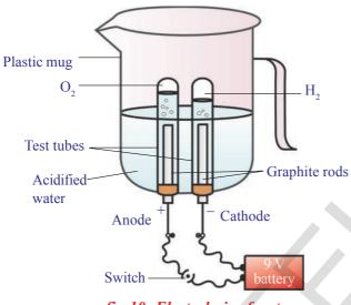
fig-10: Electrolysis of water
