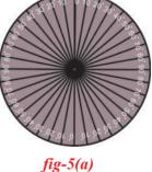
Adjust one of the straws to make an angle  $10^{\circ}$ . Immerse half of the disc vertically into the water, filled in a transparent vessel. While dipping, verify that the straw at  $10^{\circ}$  is inside the water. From the top of the vessel try to view the straw which is inside the water as shown in figure 5(b). Then adjust the other straw which is outside the water until both straws appear to be in a single straight line.
