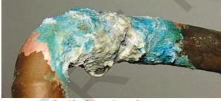
fig-18: Corrosion of copper  $2Cu + O_2 \rightarrow 2CuO \dots (38)$
