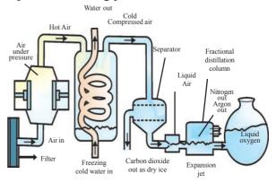
Fig-15: Separation of componants of air
