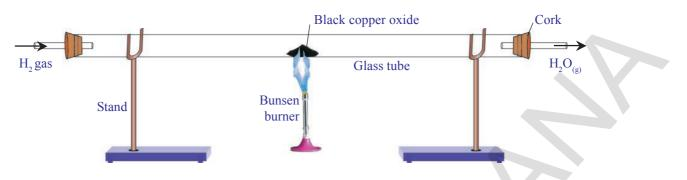
fig-16: Reduction of copper oxide to copper
