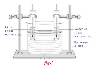
test tubes with single-holed corks. One of them is filled with 50g of water and the other with 50g of oil, both at room temperature. Insert two thermometers through holes of the corks, one each into two test tubes. Now clamp them to a retort stand and place them in a jar of hot water as shown in figure 2.
