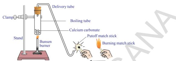
fig-8: Heating of calcium carbonate and testing the gas evolved with burning match stick
