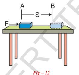
Let us assume that an object of mass (m) is at rest on a smooth horizontal plane as shown in figure 12. Let it be displaced through a distance 's' from the point A to B by a force (F) acting upon it in the direction of the displacement. In the horizontal direction the net force  $F_{net}$  is equal to the applied force F.
