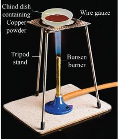
fig-15(b): Oxidation of copper to copper oxide
