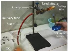
fig-9:Heating of lead nitrate and emission of nitrogen dioxide
