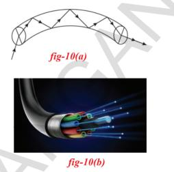
Figure 10(a) shows the principle of light transmission by an optical fibre. Figure 10(b) sketches a optical fibre cable. Because of the small radius of the fibre, light going into it makes a nearly glancing incidence on the wall. The angle of incidence is greater than the critical angle and hence total internal reflection takes place. The light is thus transmitted along the fibre.
