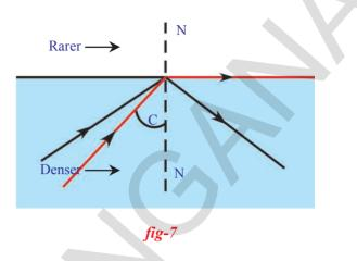
It is already found that the angle of refraction is more than angle of incidence when a light ray travels from denser $(n_1)$ to rarer medium  $(n_2)$ .
