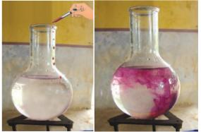
Fig - 6: Diffusion of potassium permanganate in water
