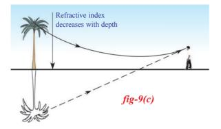
This refracted light reaches the observer in a direction shown in Figure-9c. This appears to the observer as if the ray is reflected from the ground. Hence we feel the illusion of water being present on road (shown in figure 9a) which is the virtual image of the sky (mirage) and an inverted image of tree on the road (shown in figure 9c).
