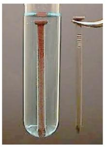
fig-13(a):Iron nail dipped in copper sulphate solution
