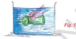
Do you feel an upward force? Try to push it further down. Do you feel any increase in the upward thrust? In fact, the upward force of water keeps on increasing as you try to push the bottle down. Now, release the bottle and observe how it bounces back to the surface of water! So the upward force of water is a real, observable force (Buoyancy). This force acting on unit area of the surface of an object (bottle) is called static pressure of the water.
