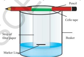
Fig-11: Separating the components of ink
